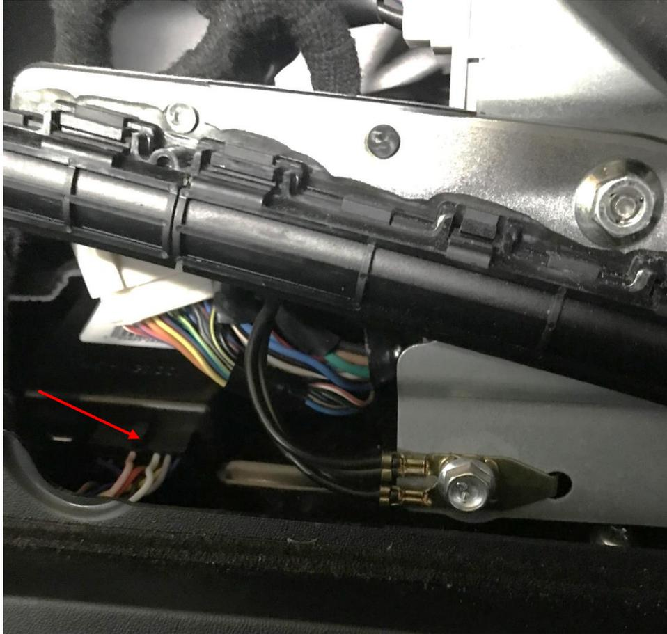
11. Turn the ignition back off, re-assemble everything, and configure the module according to our Operation and Programming manual if not configured prior to installation.
