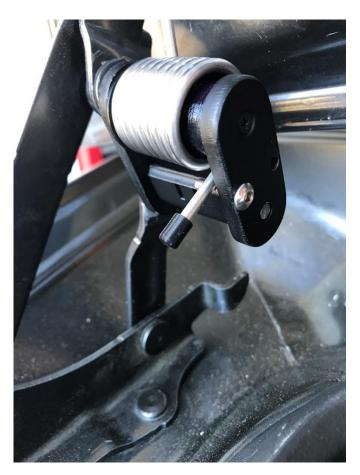
Slowly close the trunk lid and observe if there's any obstruction when closing. Once you've verified that the trunk closes correctly (with no obstructions), close it normally, which may require a little more force. Open the trunk with the key or interior button, to check if it works correctly.
