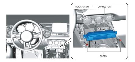
Unplug the cable from the connector. The connector has a release button on top, push down to unplug.
