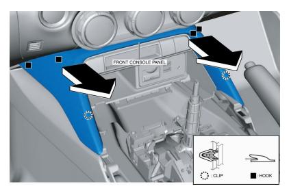
Simply pull it; it will be easier if you release the clip on one side first with help of a trim removal tool.
