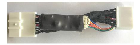
The ACC Power Controller is designed as a Plug-n-Play harness with an attached module. This module will listen to CAN messages and keep the ACC relay activated until it receives the CAN message that the driver's door is opened.
